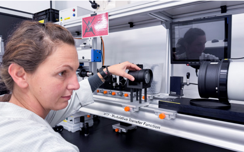
WILD staff measuring alignment errors in optics (above) and MTF measurement of lenses (left).
