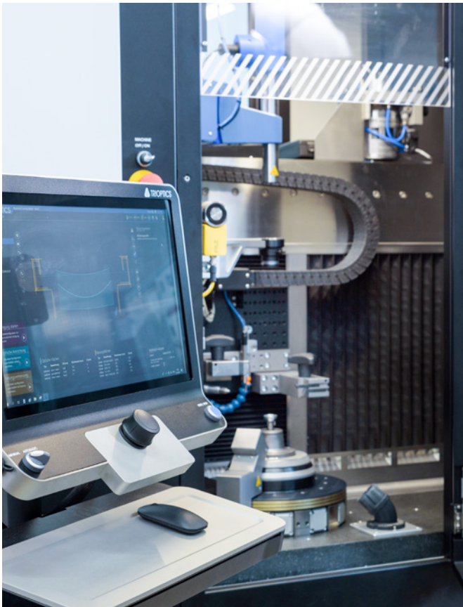
High-precision positioning of optics: Alignment turning for the highest accuracy and quality.
